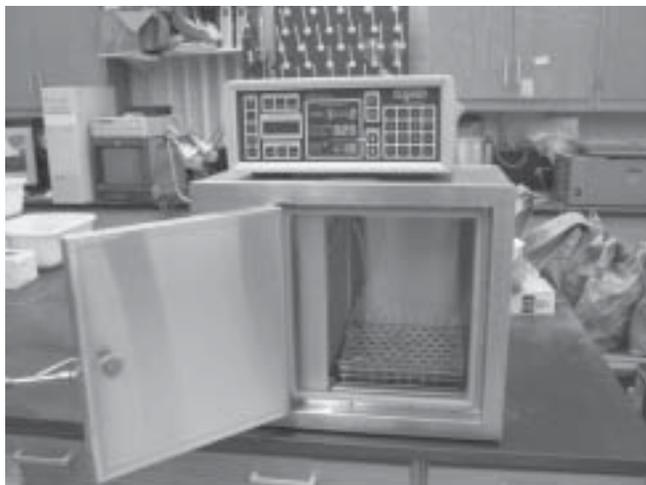
Figure 3—Cryomed freezing chamber.
