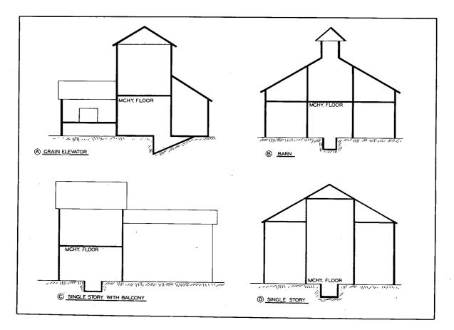
FIGURE 35.-Types of building arrangements used for seed processing plants.
