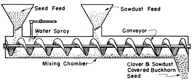
FIGURE 31.—Cross section of buckhorn machine.
