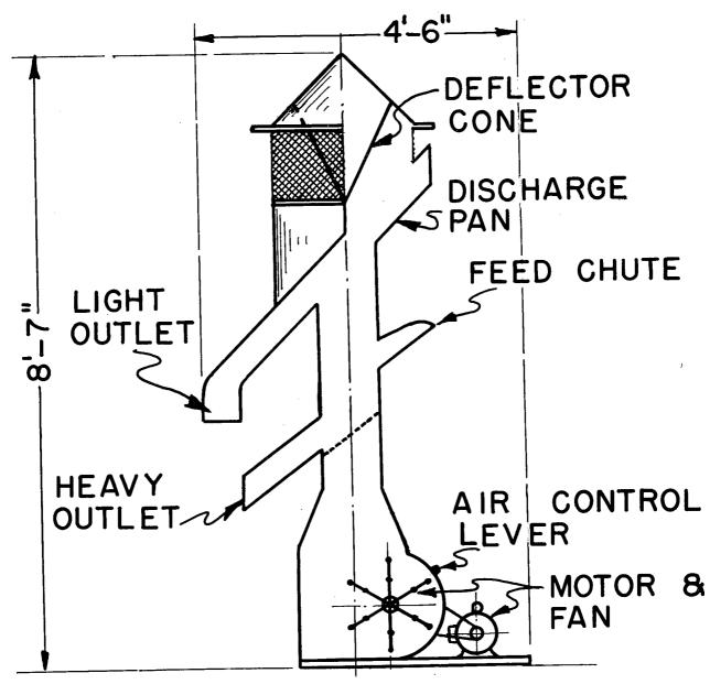
FIGURE 15.—Cross section of pneumatic separator.
