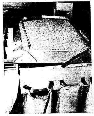
S-489-3-67 FIGURE 10.—Specific gravity separator.
