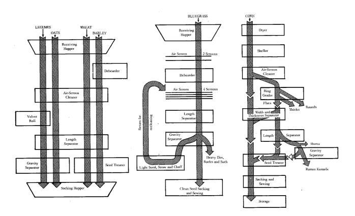
FIGURE 39.—Flow diagrams for processing seed.
