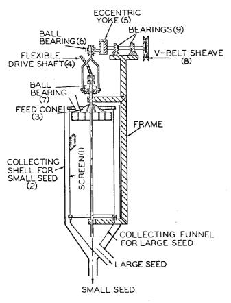
FIGURE 5.—Schematic diagram of vertical screen cylinder.
