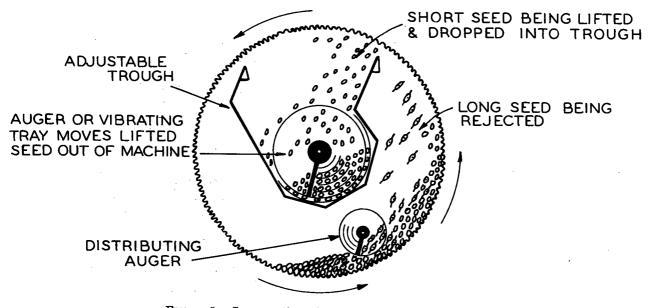
FIGURE 8.—Cross section of an indent cylinder separator.
