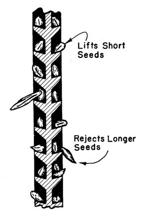
FIGURE 7.—Cross section of an indent disk separator.
