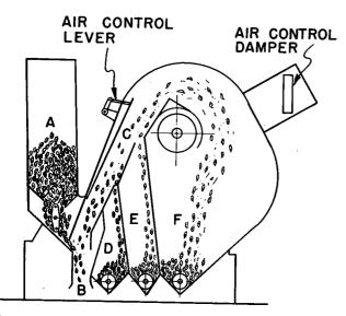
FIGURE 14.—Cross section of fractionating aspirator: A, Feed hopper; B, air column through which heavy seeds fall against the airflow; C, column into which lighter seeds and chaff are lifted; D, column which receives the heavier liftings; E, column which catches salvage grass seed, broken seed, or light and unusable seed; F, column into which extremely light waste materials are delivered.
