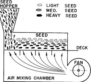
the deck may be "starved." For satisfactory separations, the deck surface should be covered at all times. An excessive feed rate will flood the deck, prevent proper stratification of the material, and cause good seeds to be discharged with the middlings or rejects.
