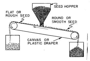
FIGURE 19.—Cross section of inclined draper seed separator.
