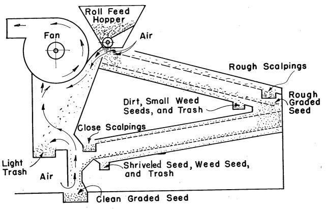
FIGURE 2.—Schematic view of air-screen cleaner.
