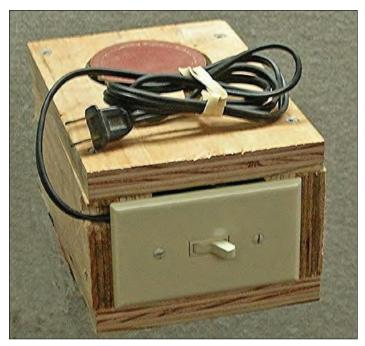
**Figure 3.** Sanding machine designed and constructed at DGRC for scarifying whitebark pine seeds before germination. (Photo by Judith Danielson, USDA Forest Service, 2009)
