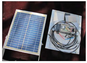
**Figure 3.** A low-cost, stand-alone, solar-powered router (both top and bottom) that uses a 2.3 Ah lead acid 12 V battery charged by a basic 10 W solar shield. The solar shield uses no costly charging regulator, only a diode to avoid battery discharge into the solar shield during the night. With the constant power demand from the radio, the battery will never be overcharged. (Photo by Daniel Girard, 2016)
