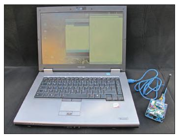
Figure 4. Receiver (stand-alone datalogger) connected to a computer to show in real time the incoming weighing data. (Photo by Daniel Girard, 2016)
