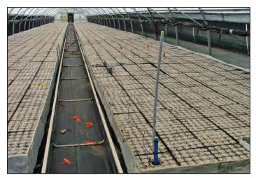
**Figure 13.** A scale (between the red flags) installed in a crop of seedlings grown in "25-310" type containers (25 cavities with a volume 310 cm<sup>3</sup> (19 in<sup>3</sup>) each, IPL 25-310 (Saint-Damien, Québec, Canada) at Grandes-Piles nursery. In front is the same antenna that was shown in figure 2. Few scales may be needed to obtain a robust statistical base for efficient irrigation management in a crop area. (Photo by Daniel Girard, 2014)
