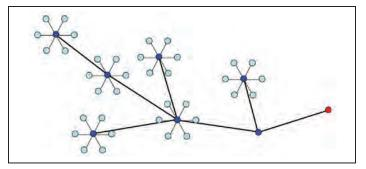
**Figure 1**. Example sketch of a wireless network (cluster tree type). Stand-alone scales (light blue) are powered by cells, and routers (deep blue) are powered using a solar shield. Each router relays the scale data in multiple hops (of no more than 200 m [610 ft] each) to expand the global network range to a single receiver (red) located at the nursery office.
