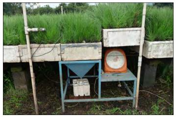
**Figure 1.** Monitoring station in a *Pinus montezumae* Lamb. seedling crop in Copperblock<sup>®</sup> 60/250ml (15 in<sup>3</sup>; Beaver Plastics Ltd., Alberta, Canada) to measure irrigation, electrical conductivity, block weight, and air temperature. (Photo by Jol Hodgson, 2012)
