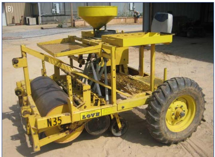
**Figure 2.** Machines used to sow a bareroot nursery (A) Vacuum precision drum sower (Silver Mountain Equipment®) and (B) Gravity drop sower (Love®). (Photos by Tom Starkey, 2009 and 2014)
