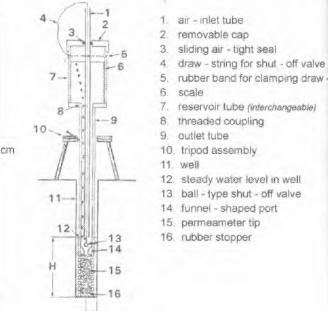
Figure 1. The head of the in-hole Mariotte-type pereameter.
