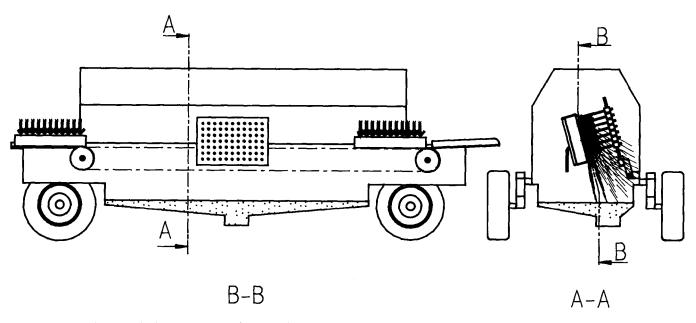
Figure 1-Tunnel sprayer, built at the Suonenjoki Research Station and Nursery, for protection against large pine weevil.
