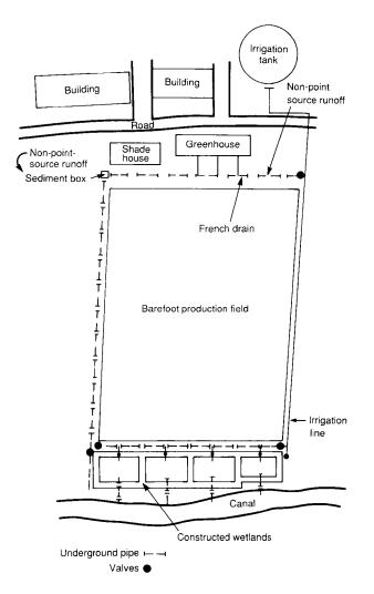
Figure 3-Overhead diagram of the constructed wetland project showing the collection area below the greenhouse complex and the location of the ponds.
