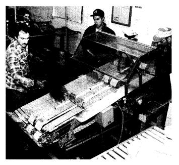
**Figure 4**—Prototype root pruner has been tested at the Forest Service's Čoeur d'Alene Nursery.
