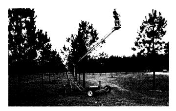
Figure 2—Highly mobile lifts make tree crown work more convenient and safer.
