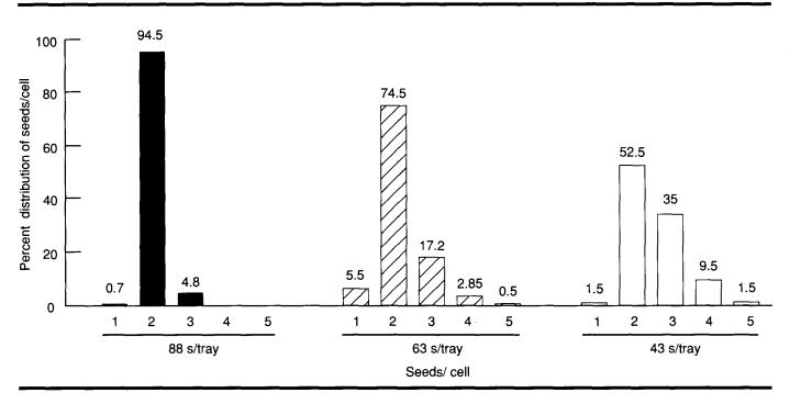
**Figure 2**—Frequency distribution of seed/cell of Douglasfir, at 3 sowing speeds (88, 63, and 43 s/tray), sown at a constant target rate of 2 seed/cell into 200-cell trays (trial 1).
