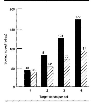
**Figure 3**—Sowing speed (s/tray) versus the target number of seed/cell for ponderosa pine (solid bars) and western larch (hatched bars) at a constant seed-supply setting of the vibrating feeder bowl (trial 2).
