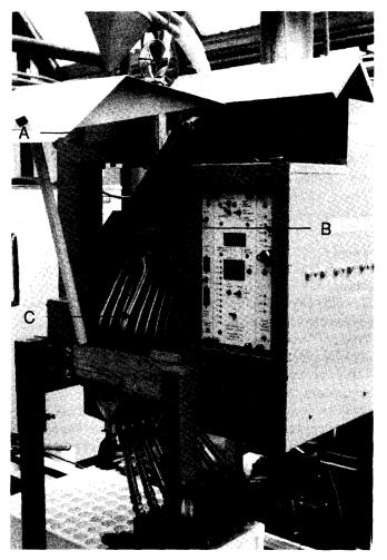
**Figure 1**—Side view of the Oldmill<sup>®</sup> optical seeder and its conveyor. A = vibratory feeder bowl, B = rotary seed distribution tube, C = upper bank of storage tubes, D = lower storage bank.
