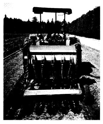
Figure 1—Ground-driven seeder sowing 5 rows of acorns.
