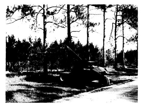
Figure 1-Conventional tree shaking operation.
