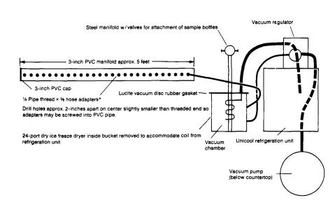
After drying the pollen for about 2 hours, screw the bottle in the adapter to seat the split stopper under vacuum. Turn the quick-seal valve off; unscrew the bottle and place a screw cap on it (the screw cap comes with the 10-ml bottle if ordered by part number 178962).
