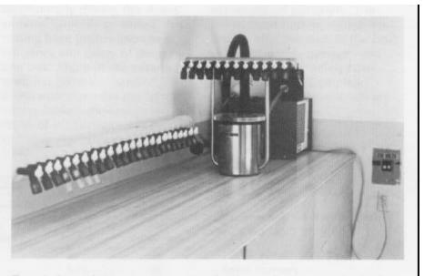
Figure 1—Freeze-drying system in use. Note that the vacuum pump is isolated below the countertop to prevent contamination of the samples with lubricating oil.
