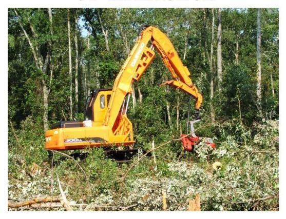
Figure 5 - Daewoo excavator with processing head.
