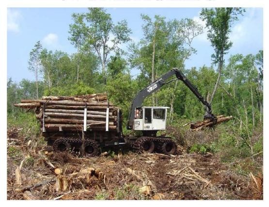
Figure 6 - Tracked forwarder collecting processed cedar logs
