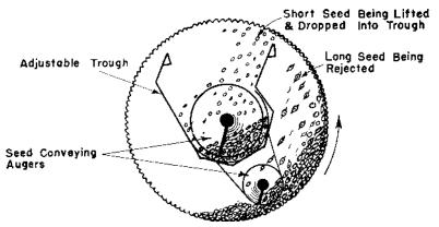
Figure 1. Cross-section view of an indent cylinder separator.
