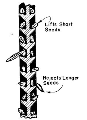
Figure 2. Cross-section view of an indent disc separator.
