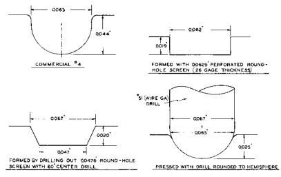
Figure 11. Indents used for removing pigweed from alfalfa.
