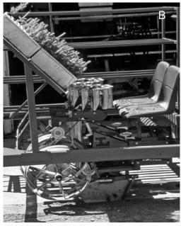
**Figure 2**—Although the MiniPlug™ Transplant System (A) proved impractical, the carousel-type transplanter (B) revived the popularity of miniplug transplants.
