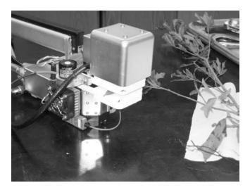
**Figure 1**—Detached leaf in leaf chamber for chlorophyll fluorescence and net photosynthesis measurements using an open gas exchange system (LI-6400; LI-COR Inc., Lincoln, NE) with an integrated fluorescence chamber head (LI-6400–40 leaf chamber fluorometer; LI-COR Inc.).
