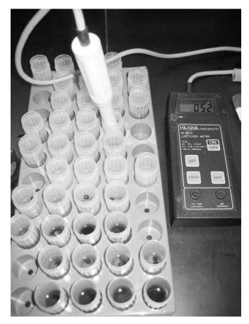
**Figure 3**—For the freeze-induced electrolyte leakage (FIEL) trial, stem and foliar samples were placed in plastic vials containing 1.5 ml (0.05 oz) water and 0.25 g (0.9 oz) sand.
