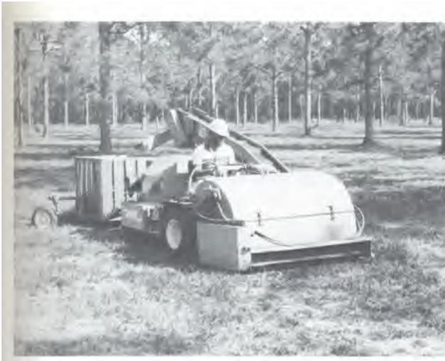
Figure 11.10. Weiss-McNair two paddle cone harvester operating in slash pine seed orchard. (Photo courtesy of Union Camp Corporation).
