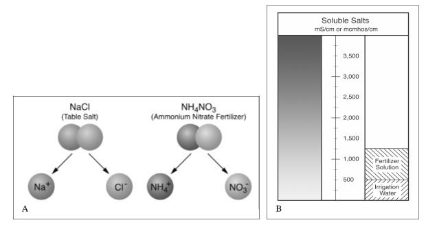
Figure 1A/B - Dissolved salts in irrigation water can be measured with electrical conductivity because they are electrically charged (A). In soil or growing media, the total salt load comes from natural sources and fertilizers (B).
