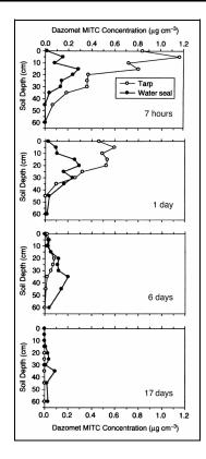
Figure 2—Recent research demonstrated that covering dazomet and metam-sodium with plastic tarps greatly increased the penetration and distribution of the gas (modified from Wang and others 2006).
