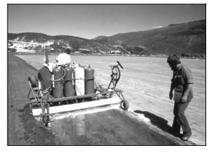
Figure 1—Plastic tarping is standard practice for methyl bromide/chloropicrin fumigation, whereas dazomet and meta-sodium fumigants are contained with a roller and water seal.
