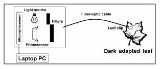
Figure 2 - A Kautsky fluorometer consists of a light source, two filters, a photosensor, a microprocessor, and a fiber-optic cable that attaches to a leaf. Instructions are sent to the fluorometer from a laptop computer.
