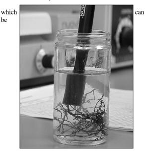
measured with a conductivity meter. The technique can be used on foliage, stem segments or root sections.
