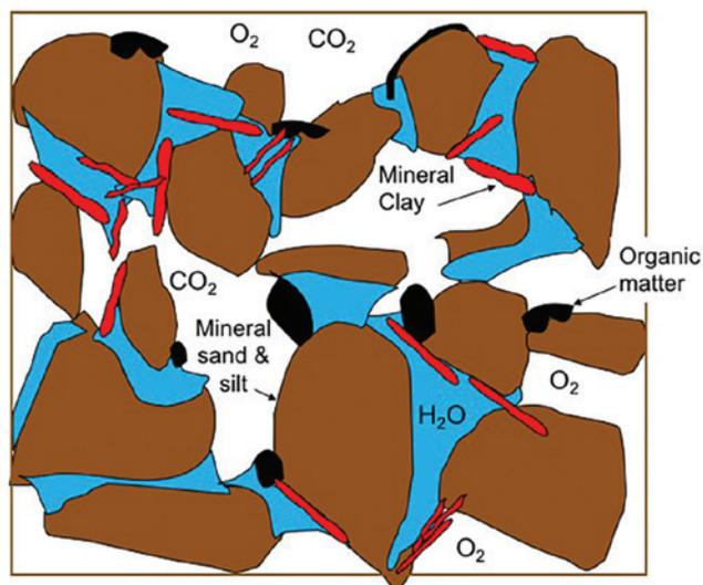
Figure 3.1—Idealized soil matrix showing inorganic and organic particles and water and air-filled pores.
