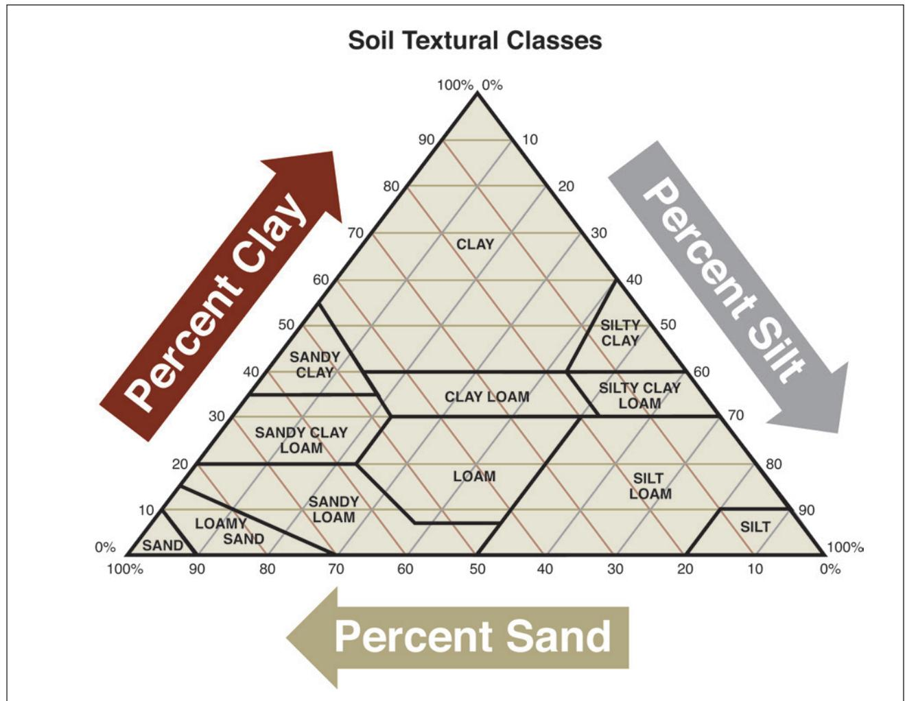
**Figure 3.2**—The soil texture triangle. Percentages of three soil particle sizes are plotted on the three axes. Texture class is determined from the percentage of any of the two groups.
