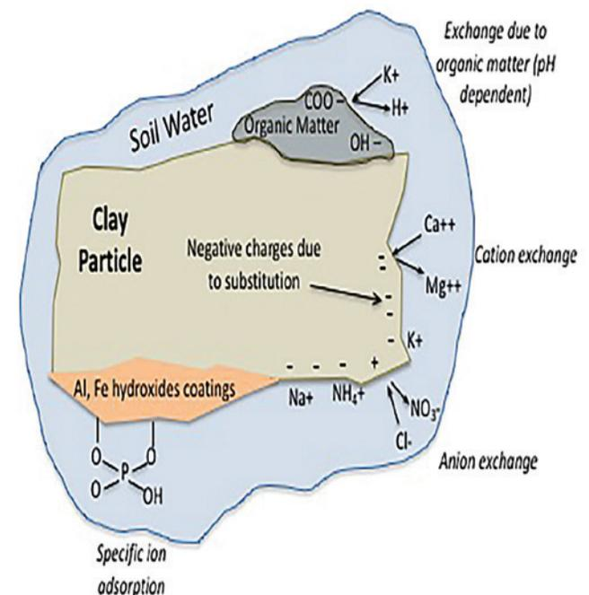
**Figure 3.6**—Adsorption and release of cations and anions on mineral and organic soil surfaces is the primary mechanism controlling availability of most essential elements.
