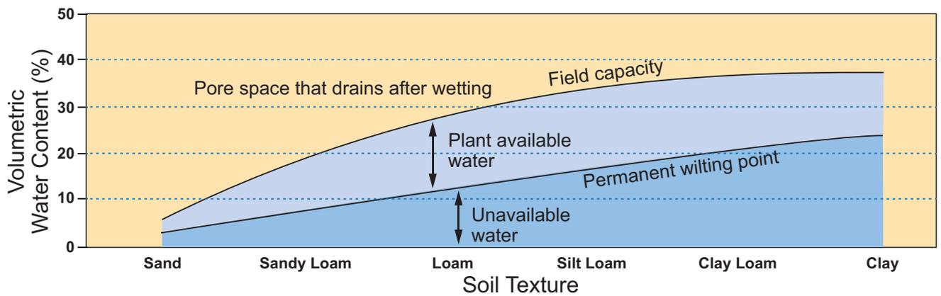
**Figure 3.4**—Water retention for noncompacted soils by soil texture class. About 50 percent of the soil is pore space. Macropores drain after rainfall and these air-filled pores are important for gas transfer. Water retained after these macropores drain is termed field capacity. Water held between field capacity and the permanent wilting point is considered plant available water.
