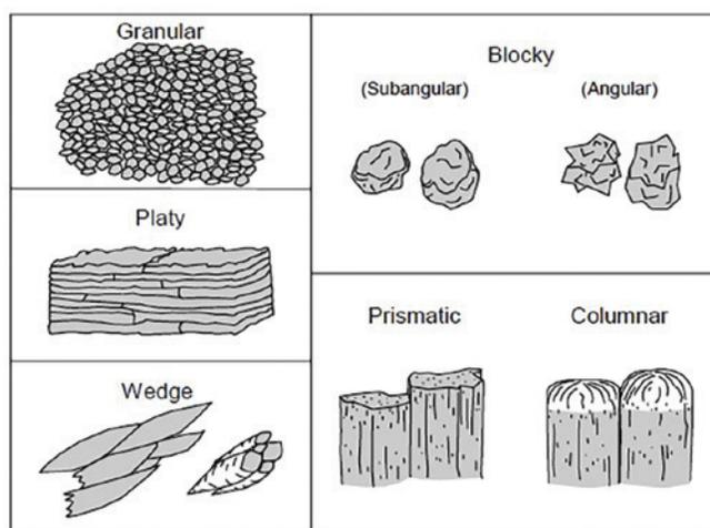
**Figure 3.3**—Individual soil particles are organized into structural units. Single-grain and granular structure are common in sandy loam and loamy textured surface soils typical of most seedling nurseries. Block structure is common in subsoils and in some nurseries with finer-textured surface soil (Schoeneberger et al. 1998).
