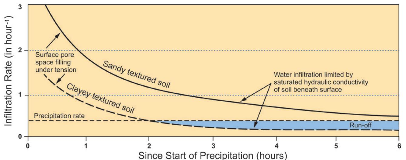
**Figure 3.5**—Response of a dry soil to precipitation. Initially, infiltration rate is high and water rapidly enters a soil under tension and fills the air-filled pore space. As the soil continues to wet and air-filled pores fill with water, the ability of the saturated soils to transmit water deeper into the profile begins to control infiltration rate.
