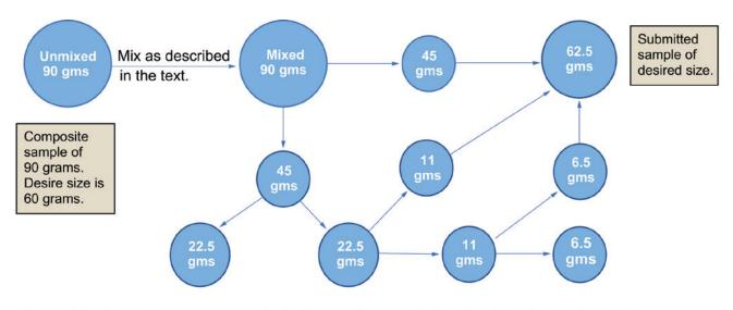
Flow of material using the correct procedure for reducing a composite sample to the desired weight for a submitted sample.
