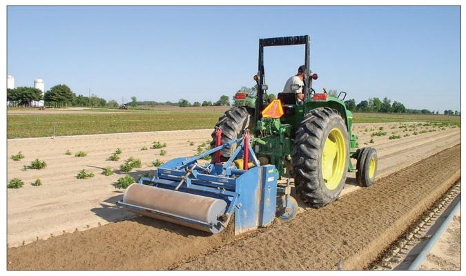
*Figure 4a.2*—Bedformers have soil rototilling functions in addition to the formation of a specific bed width. (Photo by Jeanie Redicker, Indiana Department of Natural Resources, 2013.)
