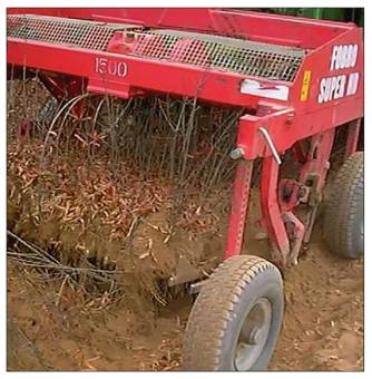
*Figure 11c.1*—Fobro lifter showing the back tine tilt angle and height above bed. (Photo courtesy of Chase Weatherly, 2017.)
