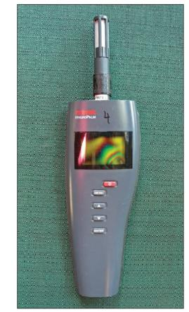
*Figure 2.19*—Handheld hygrometer for measuring equilibrium relative humidity of a seed lot. (Photo by R. Karrfalt, USDA Forest Service.)
