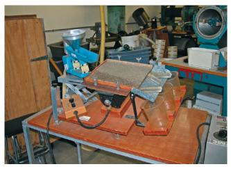
**Figure 2.17**—The vibratory separator removes trash from seeds by differences in surface texture. (Photo by R. Karrfalt, USDA Forest Service.)
