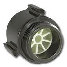
**Figure 5.3**—Sprinkler nozzle with stream straightener vanes installed. A sprinkler's throw distance will be increased by 3 to 4 feet (.9 to 1.2 m) and the application uniformity will be greater if the streamlines exiting the sprinkler nozzles are straight. (Photo courtesy of Irrigation-Mart. 2011.)
