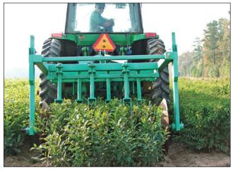
*Figure 11d.8*—Whitfield<sup>®</sup> lateral pruner over sawtooth oak. (Photo by R. Cross.)
