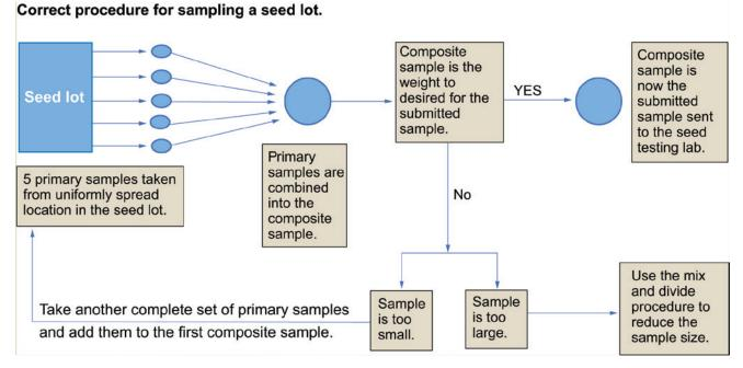
Figure 2.23—Flow of work in sampling a seedlot for testing its quality.
