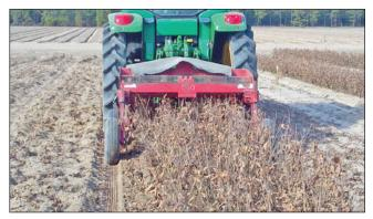
*Figure 11d.9*—*Fobro*<sup>®</sup> *Lifter. (Photo by R. Cross.)*
