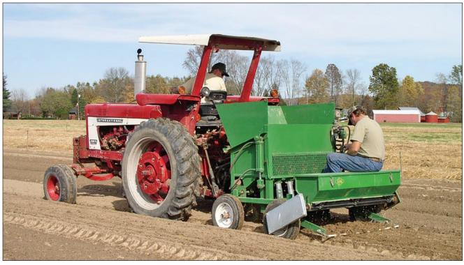
**Figure 4a.4**—Operation of a large acorn seeder. This seeder was built at the Vallonia State Nursery in Indiana. A living mulch seed sower attached to the back of the acorn sower sows wheat, rye, or oats simultaneous to acorns. (Photo by Jeanie Redicker, Indiana Department of Natural Resources, 2013.)
