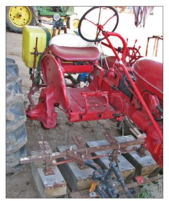
**Figure 8b.6**—This photograph shows an example of a shielded herbicide applicator designed for hardwood seedbeds. The advantage of this model is that it can be operated by one person. (Photo by David South, 2010.)
