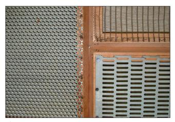
**Figure 2.11**—Hand screens showing the three main types of screens used to clean seedlots (counter-clockwise from left): perforated metal round hole, perforated metal oblong holes, and woven wire. (Photo by R. Karrfalt, USDA Forest Service.)
