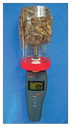
**Figure 2.20**—A recycled peanut butter jar used as a test chamber for measuring equilibrium relative humidity (eRH) to test if the seed is dry for storage. A 30-percent eRH is good for all seeds that should be dried. (Photo by R. Karrfalt, USDA Forest Service.)
