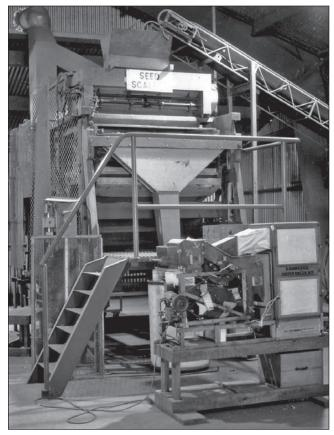
*Figure 2.12*—*Air-screen machines come in many sizes and are used for basic seed cleaning; a small cleaner is in front of a very large cleaner. (Photo by R. Karrfalt, USDA Forest Service.)*
